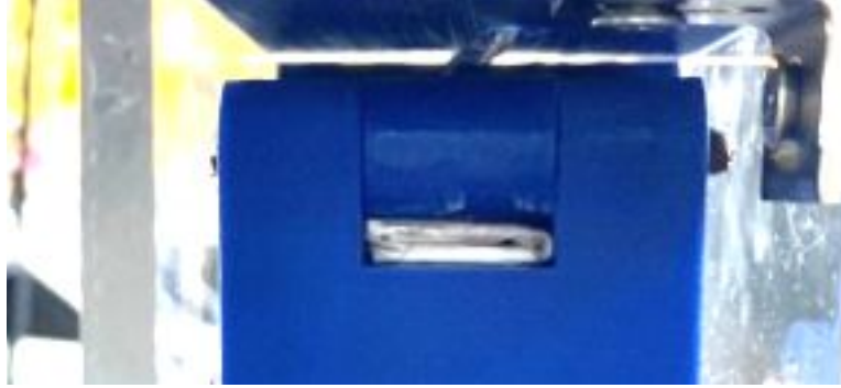
Figure 13. Glued padding added to restrict top arm rotation
