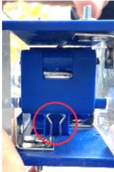
Figure 18. Binder clip attached
